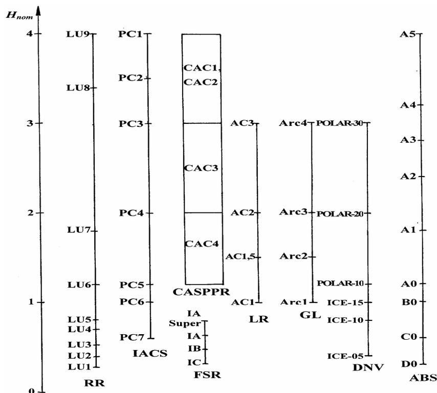
Fig. 4. The equivalent ice thickness  $H_{nom}$  related to different ice classes (Appolonov et al. 2007).
