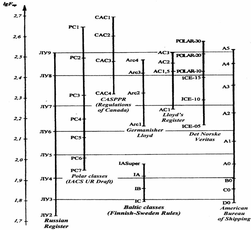
Fig. 5. Comparison between different ice classes based on hull weight (Appolonov et al. 2007).
