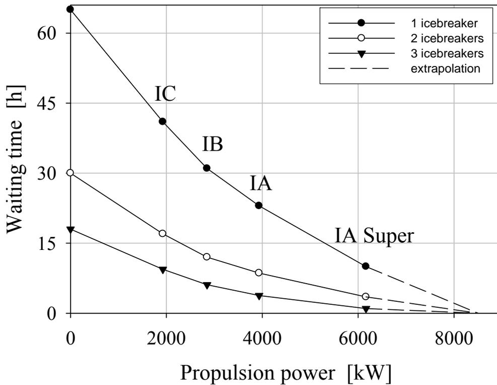
Fig. 1. The waiting times for an icebreaker in a winter navigation system modified from the Estonian system shown in terms of propulsion power and using the number of icebreakers as a parameter. The propulsion power '0' refers to open water ships that cannot sail in ice at all. The Figure corresponds to ice conditions in a severe winter.
