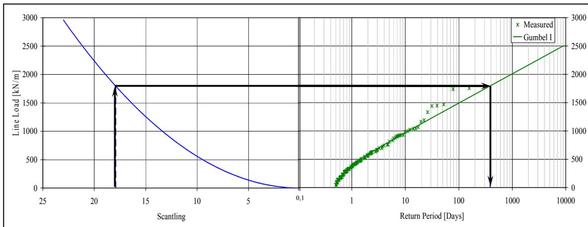
Fig. 2. Estimation of the risk level for a given ship (from scantlings to the frequency of the defined ice damage). The direction of arrows may be reversed, proceeding from a certain load frequency through a preset damage to scantlings (SAFEICE, D9-2).
