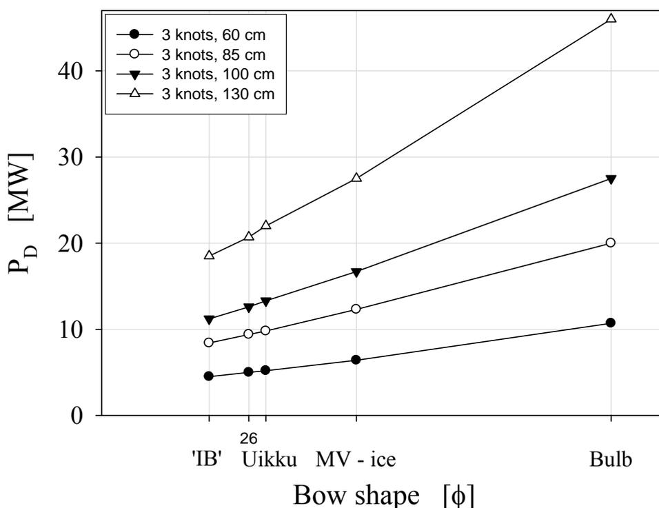
Fig. 3. The propulsion power requirement for ship versions defined in this report in different ice thicknesses.
