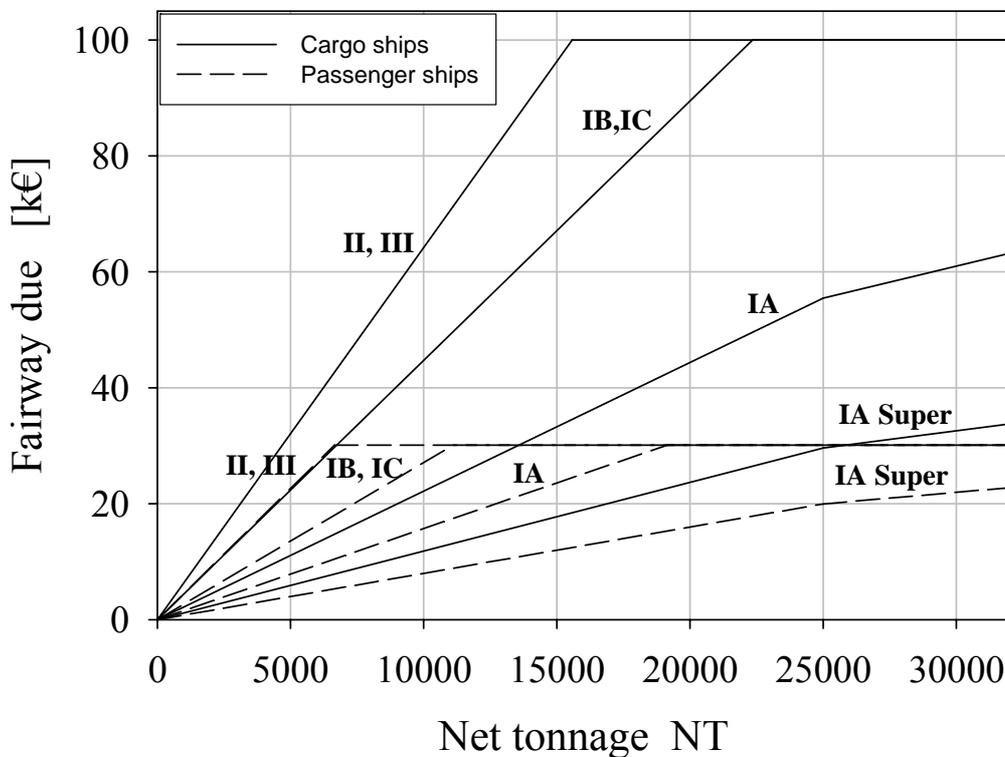
Fig. 6. The fairway dues of ships with the ice class as a parameter. The lowest broken line for both ship types corresponds to ice class IA Super, and the lines above that ice classes IA, IB and IC both II and III.
