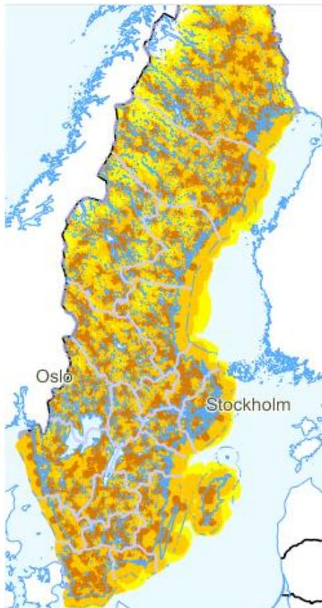
*Figure 4. Coverage area using 450 MHz network offered by the Swedish operator Net 1. Yellow area is the coverage using external antenna.*
