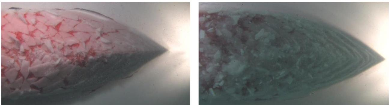
Figure 5-2: Underwater footage. Left = 0.69 m/s (6 kn); right = 1.38 m/s (12 kn). The bow is considerably covered in ice at 1.38 m/s speed.
