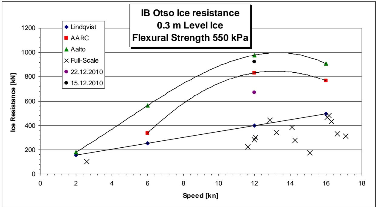
Figure 7-1: The measured ice resistances of all tests. A turbulence stimulator is used at 15.12.2010 and 22.10.2010.
