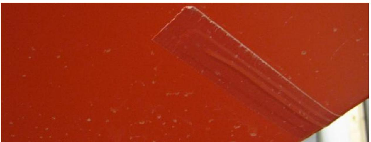
*Figure 2-6: The turbulence simulator was made from a welding wire which had two layers of tape above it. The first tape layer was half of the width of the second.*
