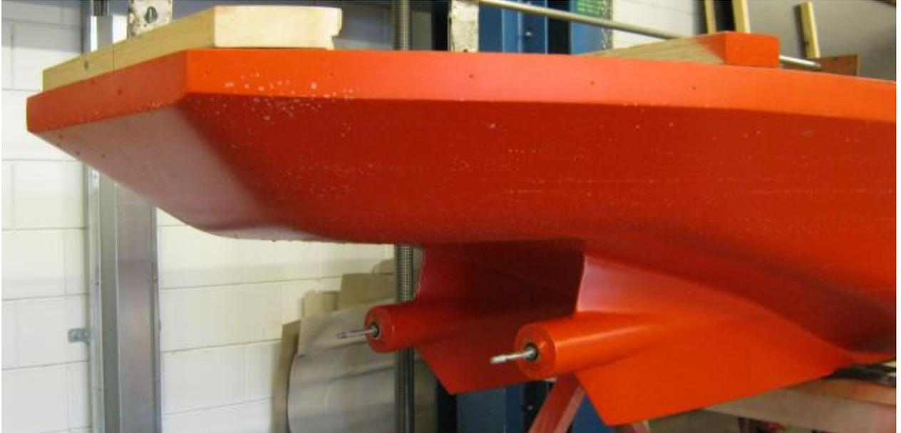
Figure 2-2: The stern of the model. No propellers were used.
