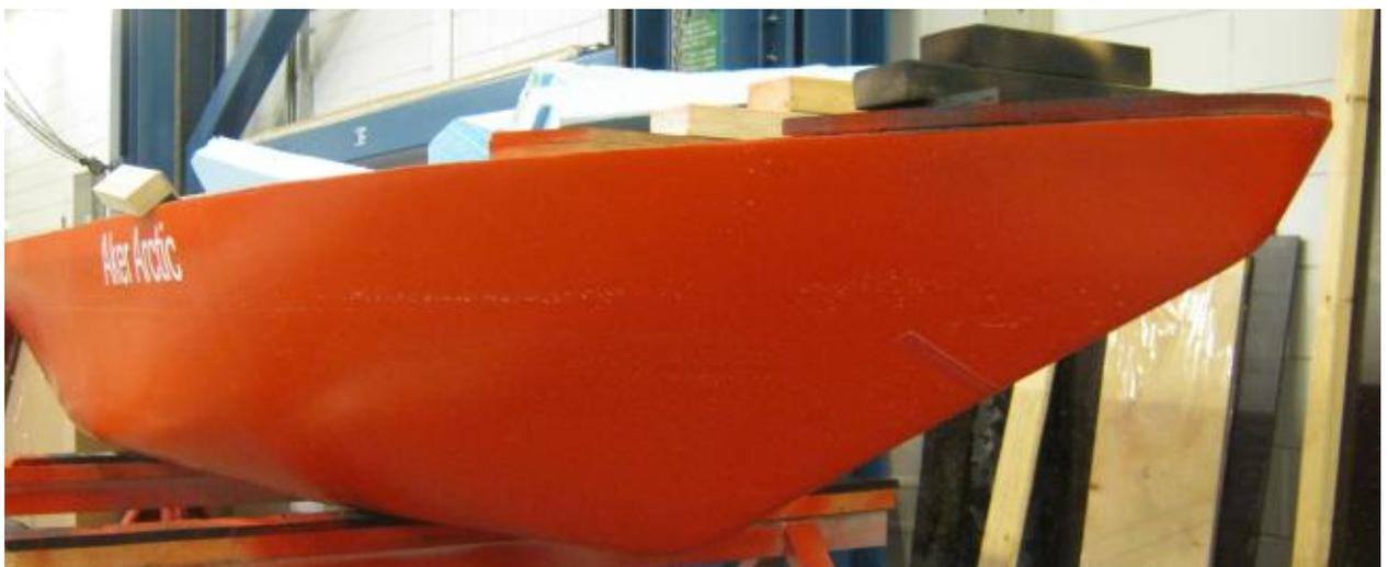
Figure 2-1: The bow of the model. The turbulence stimulator is intact on the bow.
