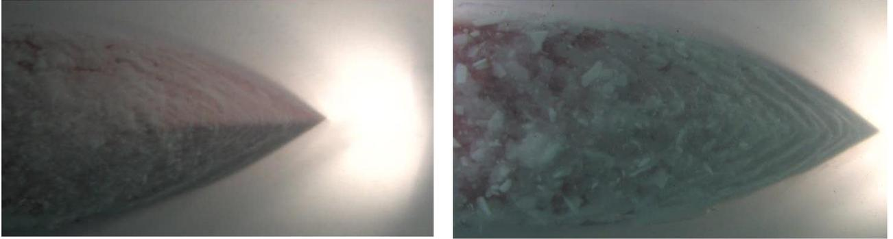
Figure 6-1: Underwater footage. Left =turbulence stimulator; right = original hull.
