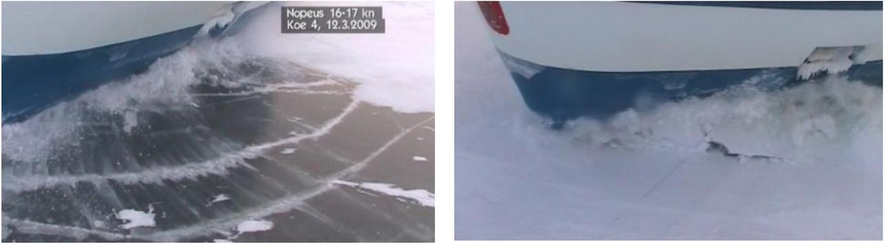
*Figure 4-3: Ice breaking in full scale at high speed.*
