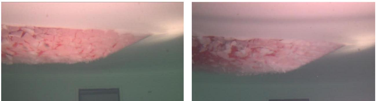
*Figure 5-3: Underwater footage. Left = 0.69 m/s; right = 1.38 m/s. Small waves of crushed ice can be seen above the ice layer in the right picture.*
