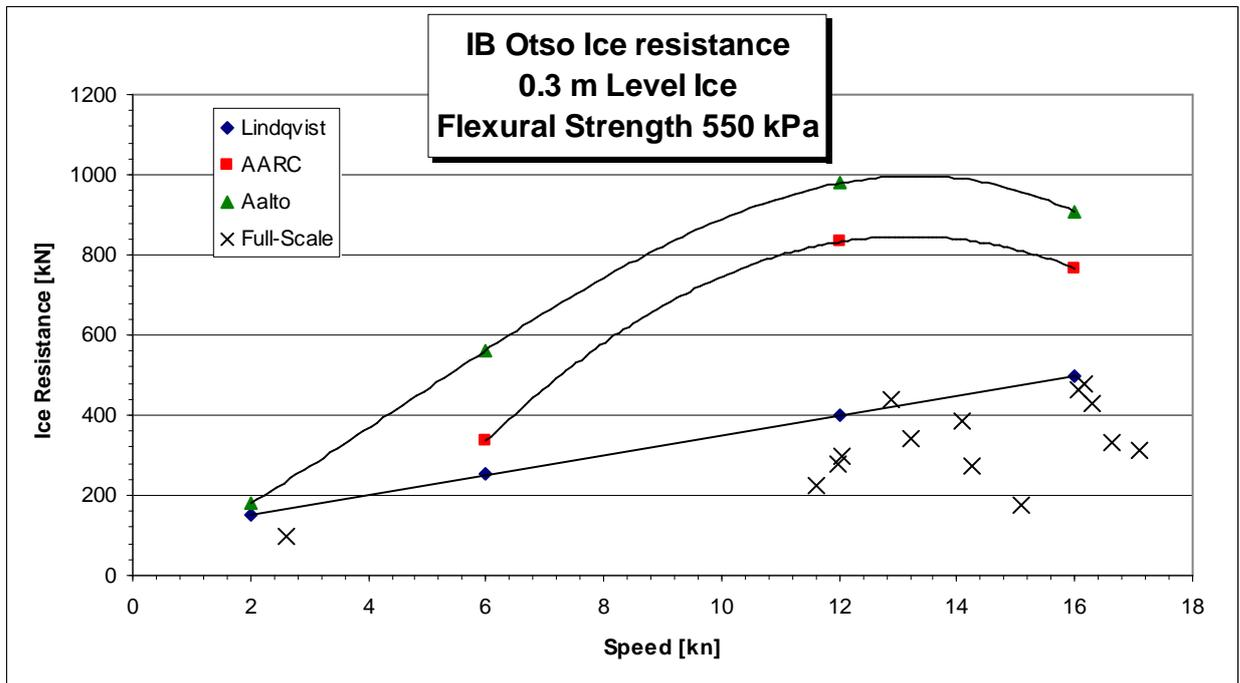
Figure 5-1: The measured ice resistance for IB Otso.
