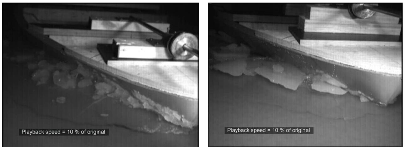
Figure 4-2: Breaking the ice at 1.84 m/s. Left = less saline ice; right = normal model ice.
