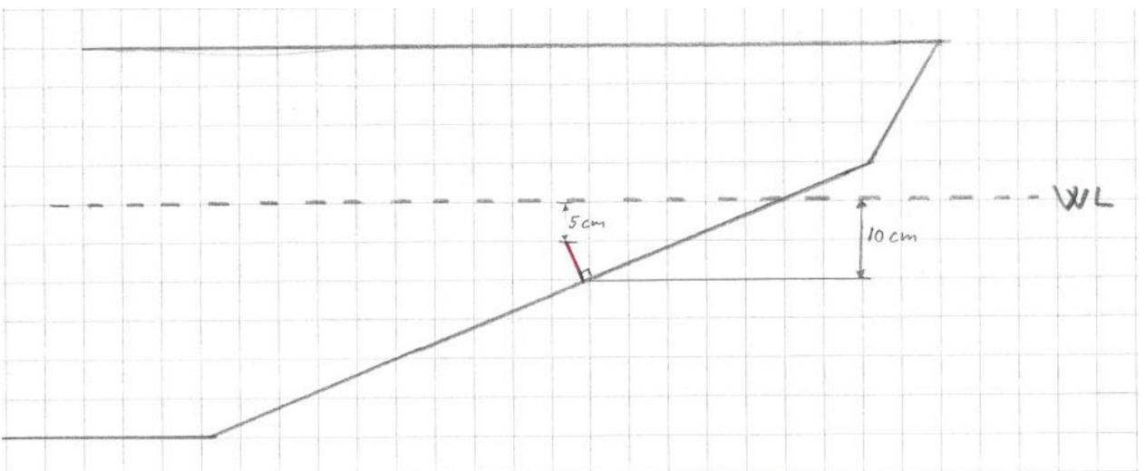
Figure 2-4: The position of the turbulence stimulator (marked with a red line). The picture is not in scale.
