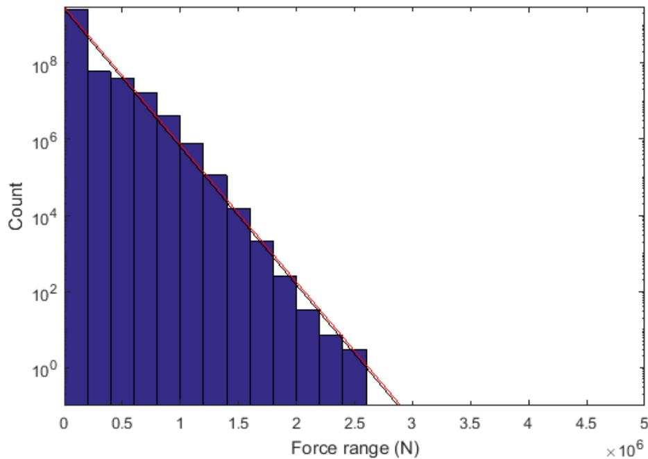
Figure 8. The modelled force ranges at the thruster strut for ship 3 without any dynamic magnification of blade loads ( $C_{DM1}$  in Table 5 used). The black curve is Weibull distribution with a shape factor 1, and the maximum ice load and the number of loads are taken from the model results. The red curve is Weibull distribution with the values taken from the guidelines of FSICR.
