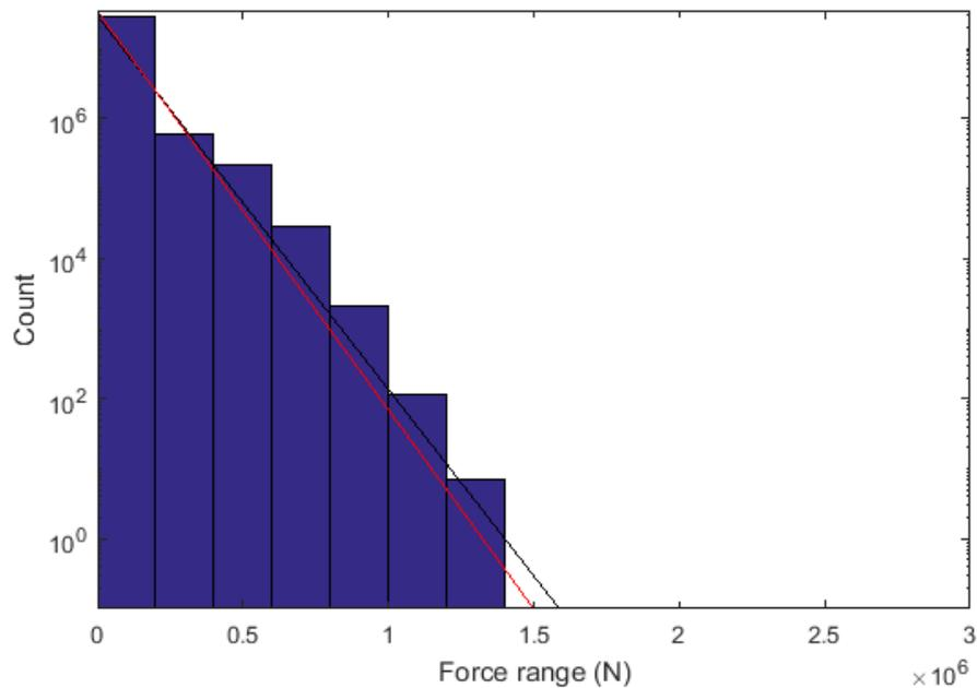
Figure 11. The modelled force ranges at the thruster strut for ship 4 without any dynamic magnification of blade loads ( $C_{DM1}$  in Table 5 used). The black curve is Weibull distribution with a shape factor 1, and the maximum ice load and the number of loads are taken from the model results. The red curve is Weibull distribution with the values taken from the guidelines of FSICR.
