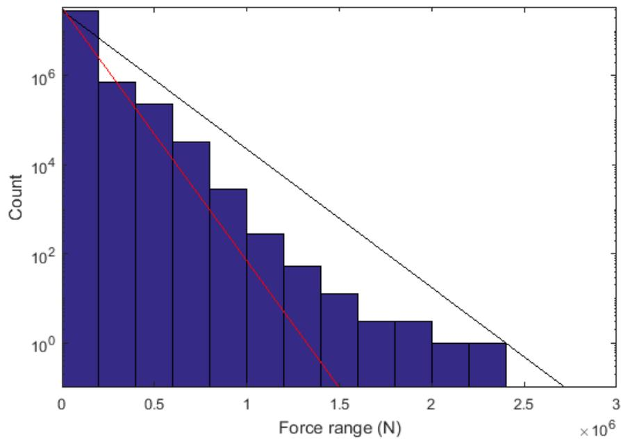
Figure 12. The modelled force ranges at the thruster strut for ship 4 with dynamic magnification of blade loads at intermediate power levels ( $C_{DM2}$  in Table 5 used). The black curve is Weibull distribution with a shape factor 1, and the maximum ice load and the number of loads are taken from the model results. The red curve is Weibull distribution with the values taken from the guidelines of FSICR.
