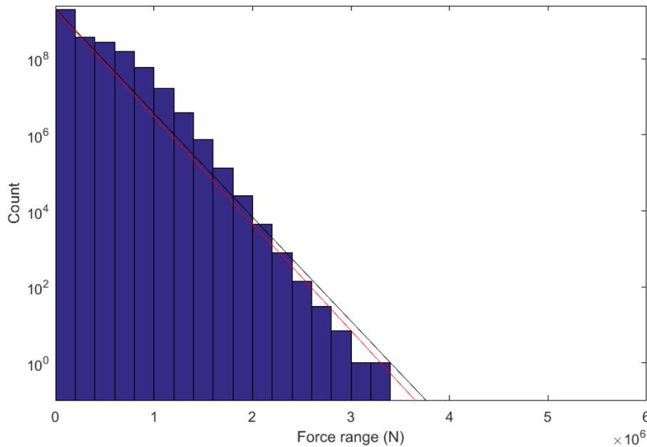
Figure 2. The modelled force ranges at the thruster strut for ship 1 without any dynamic magnification of blade loads ( $C_{DM1}$  in Table 5 used). The black curve is Weibull distribution with a shape factor 1, and the maximum ice load and the number of loads are taken from the model results. The red curve is Weibull distribution with the values taken from the guidelines of FSICR.
