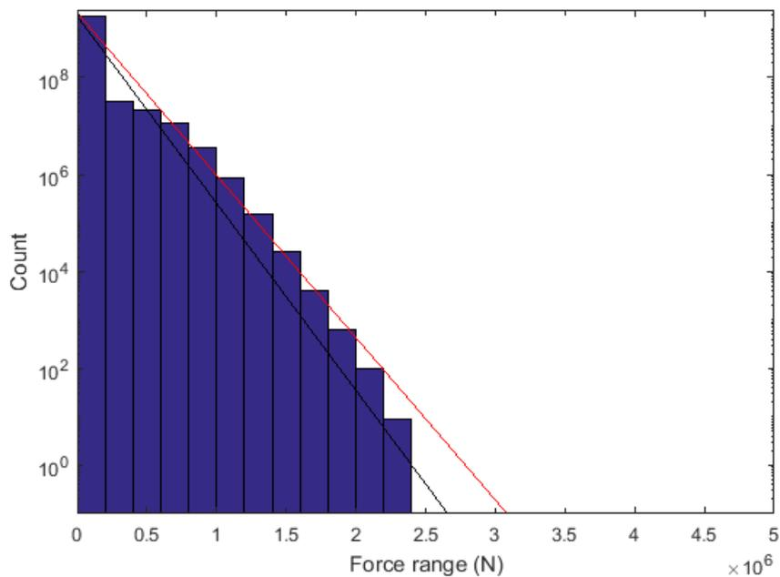
Figure 5. The modelled force ranges at the thruster strut for ship 2 without any dynamic magnification of blade loads ( $C_{DM1}$  in Table 5 used). The black curve is Weibull distribution with a shape factor 1, and the maximum ice load and the number of loads are taken from the model results. The red curve is Weibull distribution with the values taken from the guidelines of FSICR.
