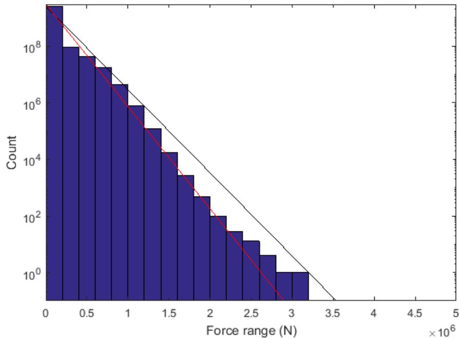
Figure 10. The modelled force ranges at the thruster strut for ship 3 with dynamic magnification of blade loads at high power levels ( $C_{DM3}$  in Table 5 used). The black curve is Weibull distribution with a shape factor 1, and the maximum ice load and the number of loads are taken from the model results. The red curve is Weibull distribution with the values taken from the guidelines of FSICR
