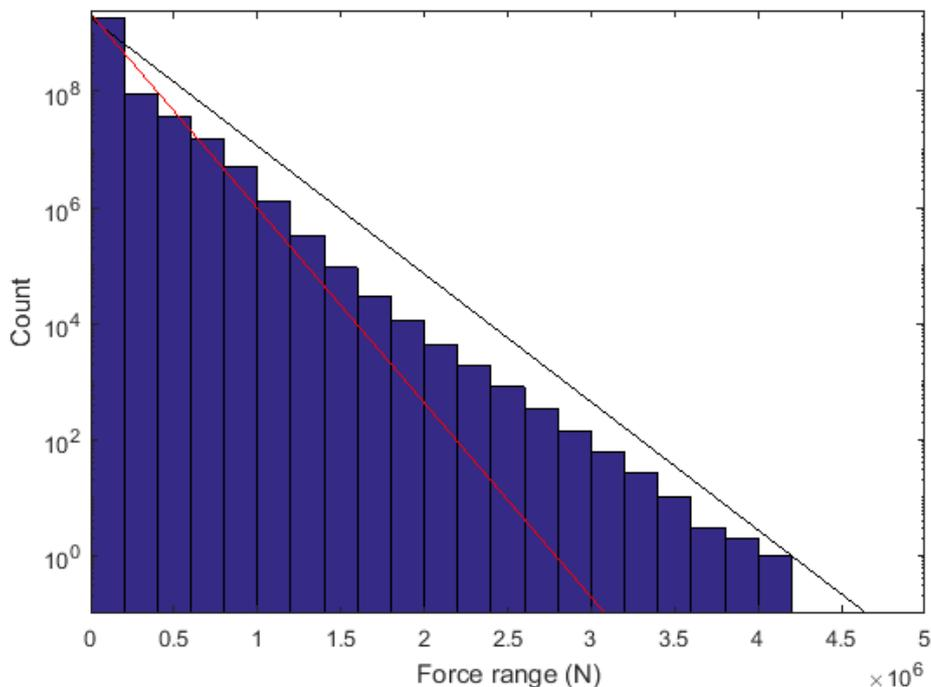
Figure 7. The modelled force ranges at the thruster strut for ship 2 with dynamic magnification of blade loads at high power levels ( $C_{DM3}$  in Table 5 used). The black curve is Weibull distribution with a shape factor 1, and the maximum ice load and the number of loads are taken from the model results. The red curve is Weibull distribution with the values taken from the guidelines of FSICR.
