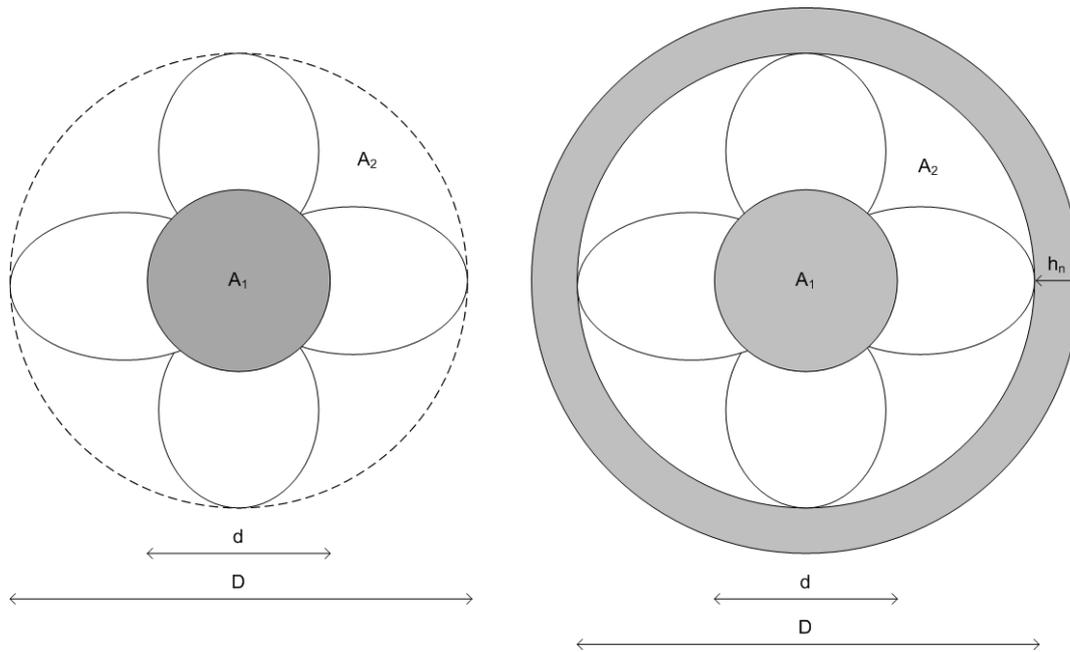
Figure 1. Schematic cross-sections of open (left) and ducted propeller (right). The grey area shows the places where ice impact is delivered straight to the thruster hull structure and the white area shows the area where ice impacts to blades.
