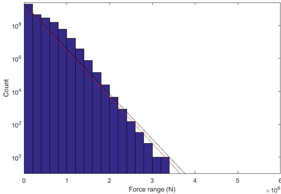
Figure 4. The modelled force ranges at the thruster strut for ship 1 with dynamic magnification of blade loads at high power levels ( $C_{DM3}$  in Table 5 used). The black curve is Weibull distribution with a shape factor 1, and the maximum ice load and the number of loads are taken from the model results. The red curve is Weibull distribution with the values taken from the guidelines of FSICR.
