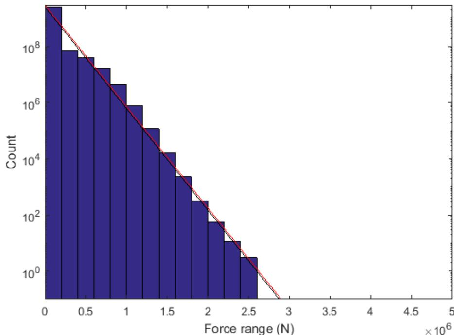
Figure 9. The modelled force ranges at the thruster strut for ship 3 with dynamic magnification of blade loads at intermediate power levels ( $C_{DM2}$  in Table 5 used). The black curve is Weibull distribution with a shape factor 1, and the maximum ice load and the number of loads are taken from the model results. The red curve is Weibull distribution with the values taken from the guidelines of FSICR.
