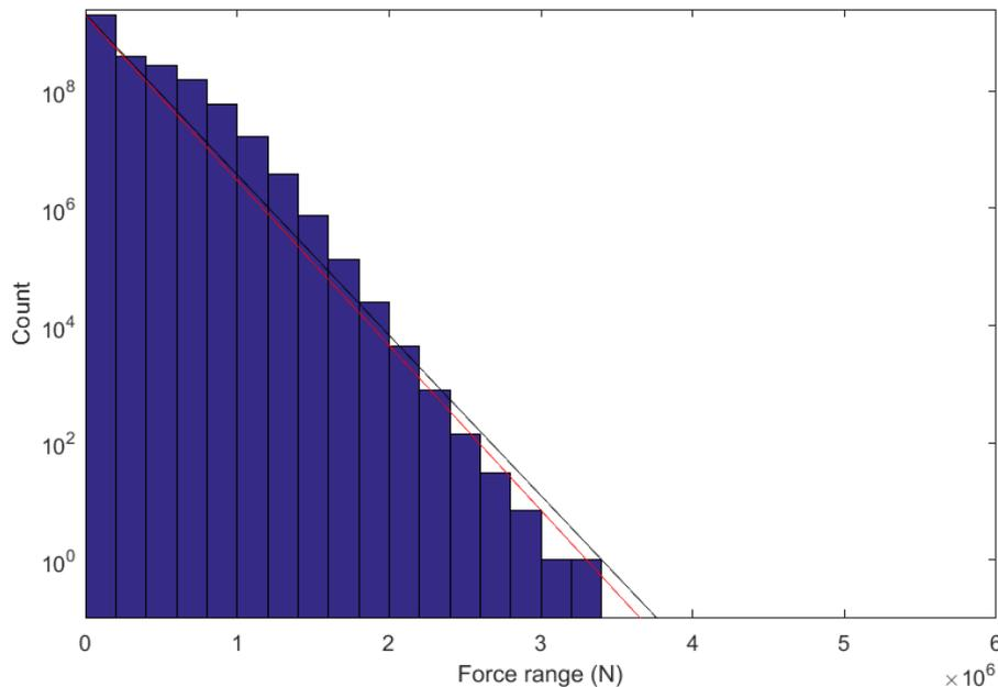
Figure 3. The modelled force ranges at the thruster strut for ship 1 with dynamic magnification of blade loads at intermediate power levels ( $C_{DM2}$  in Table 5 used). The black curve is Weibull distribution with a shape factor 1, and the maximum ice load and the number of loads are taken from the model results. The red curve is Weibull distribution with the values taken from the guidelines of FSICR.
