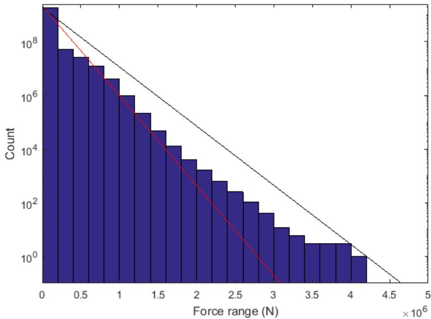
Figure 6. The modelled force ranges at the thruster strut for ship 2 with dynamic magnification of blade loads at intermediate power levels ( $C_{DM2}$  in Table 5 used). The black curve is Weibull distribution with a shape factor 1, and the maximum ice load and the number of loads are taken from the model results. The red curve is Weibull distribution with the values taken from the guidelines of FSICR.
