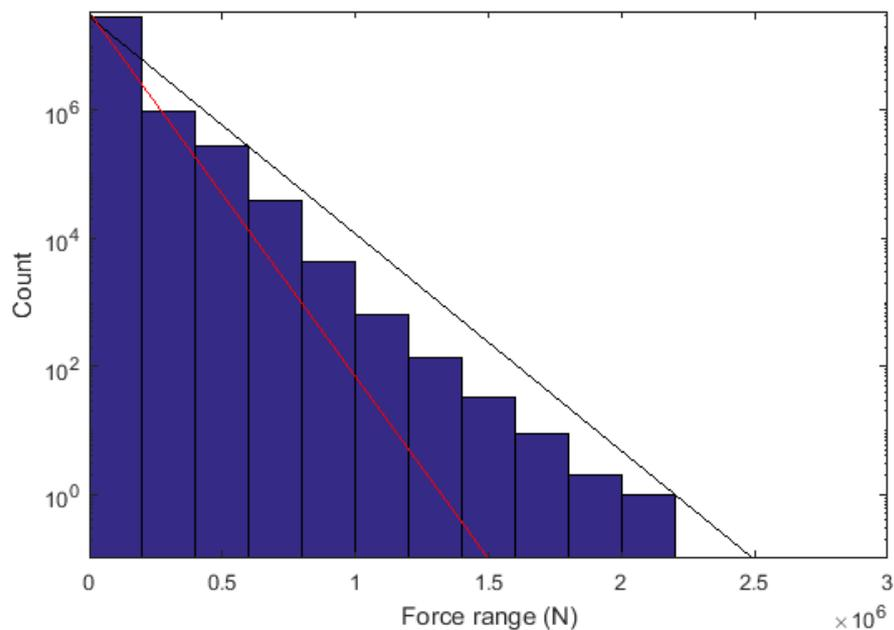
Figure 13. The modelled force ranges at the thruster strut for ship 4 with dynamic magnification of blade loads at high power levels ( $C_{DM3}$  in Table 5 used). The black curve is Weibull distribution with a shape factor 1, and the maximum ice load and the number of loads are taken from the model results. The red curve is Weibull distribution with the values taken from the guidelines of FSICR.
